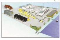
HDD is a method of installing underground utilities when trenching work is impractical to perform. The underground portion of the project will require two HDD sites along the route.
