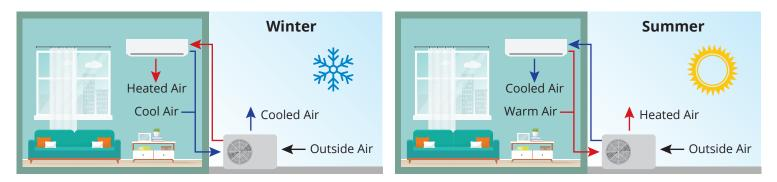
Heat pump air conditioning systems work by moving heat. Because they both heat and cool, they save energy and money over their lifetime while improving indoor air quality.
