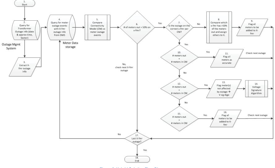
Figure 2. Hybrid Solution Flow Diagram
