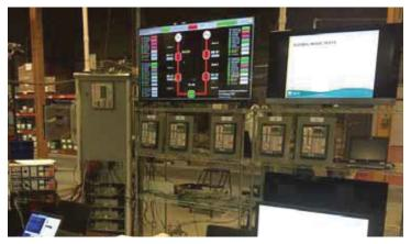
Figure 2. Test Setup for Factory Acceptance Testing
