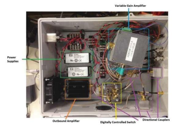
Figure 3. Coupler Peripheral Box
