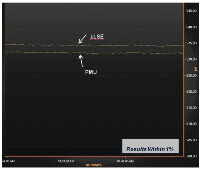
Figure 7. Lugo 500-kV West Bus Comparison
