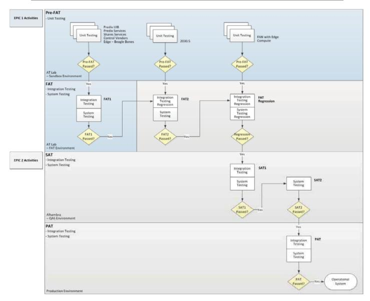
Figure 8: Overall IGP Test Approach
