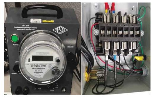
Figure 2. Meter Sockets Used for Testing
