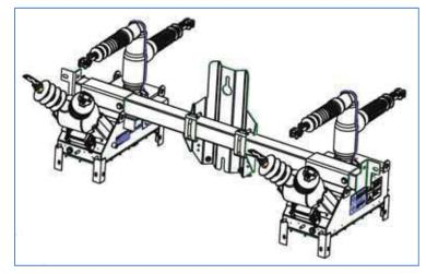
Figure 2. Intelligent Fuses Mounted on Crossarm
