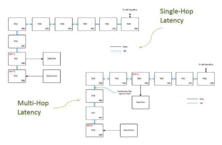
Figure 11: Radio Test Scenarios in the Performance environment
