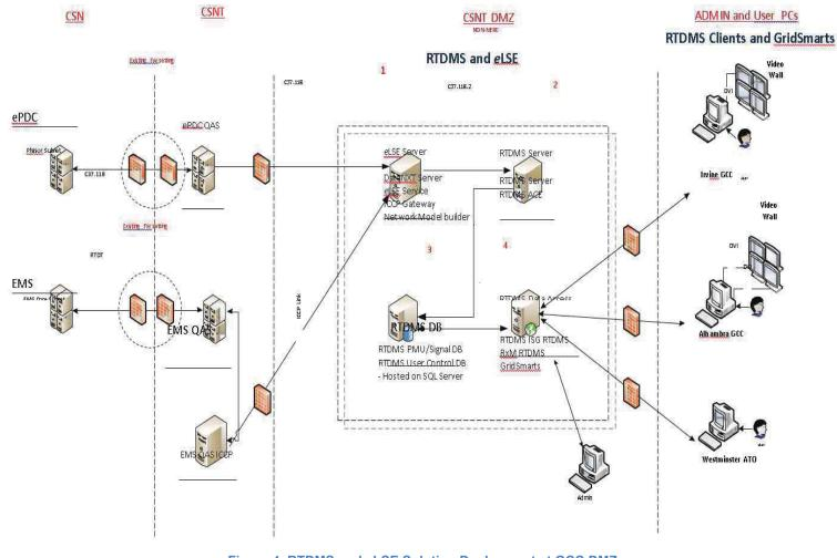
Figure 4. RTDMS and eLSE Solution Deployment at GCC DMZ
