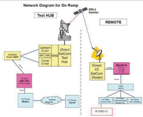
Figure 3. Network Architecture Diagram for the On-Ramp Wireless Over Satellite Integration
