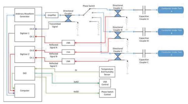
Figure 5. The HiZ Research Environment for Three-Phase Monitoring
