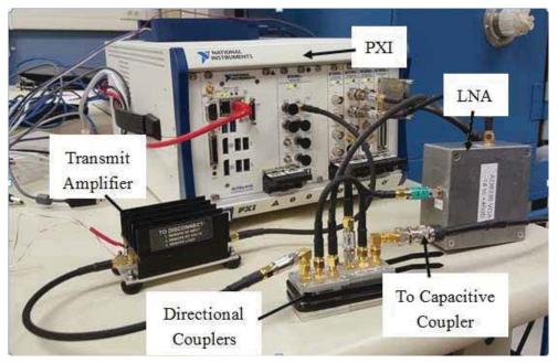
Figure 6. PXI, Coupler and Amplifier Setup
