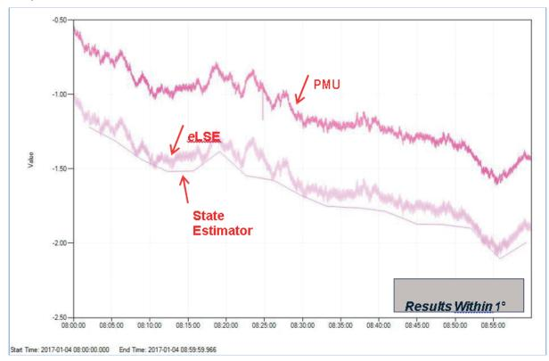
Figure 8. Vincent-Lugo 500-kV Angle Difference Comparison
