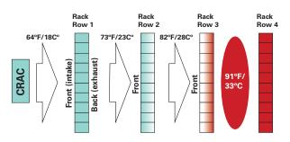
But if several rows are set up in the same orientation, the second row of racks takes in hot exhaust air from the first row. The problem is magnified with each progressive row, as the air temperature becomes hotter, causing more energy usage from A/C to keep the data center cool.
