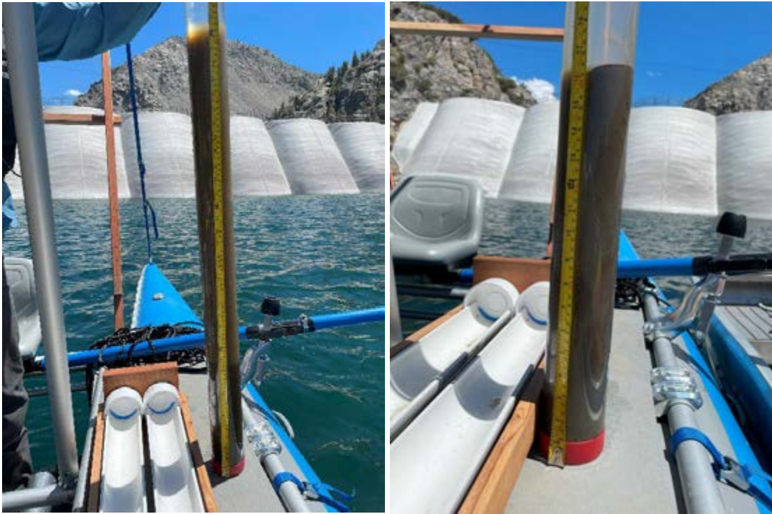
Photo B-19. Gem 5 contaminant and gradation sample extracted with plastic core sleeve.
