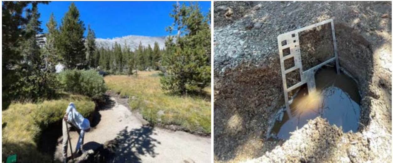
Photo B-35. Reference 3 sediment sample collected on low gradient meadow channel.
