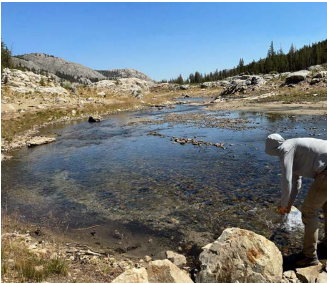
Photo A-1. Waugh 1 Sediment Sample Collected in the upstream, higher gradient, portion of channel with a stainless-steel shovel
