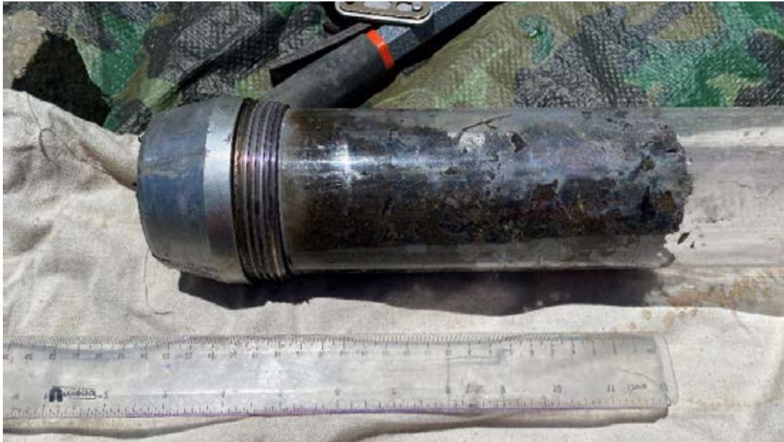
Photo B-26. Agnew 2 contaminant and gradation core sample extracted with plastic sleeve. The top 6 inches of the sample was composed of organic matter.
