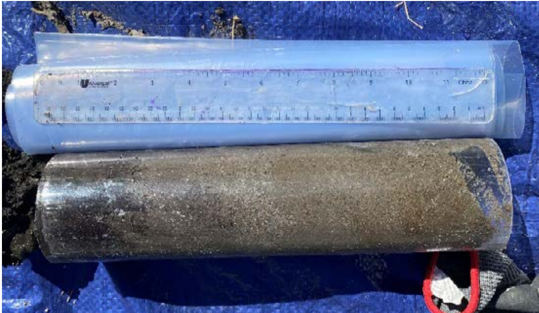
Photo B-24. Agnew 1 contaminant and gradation core sample extracted with plastic sleeve.
