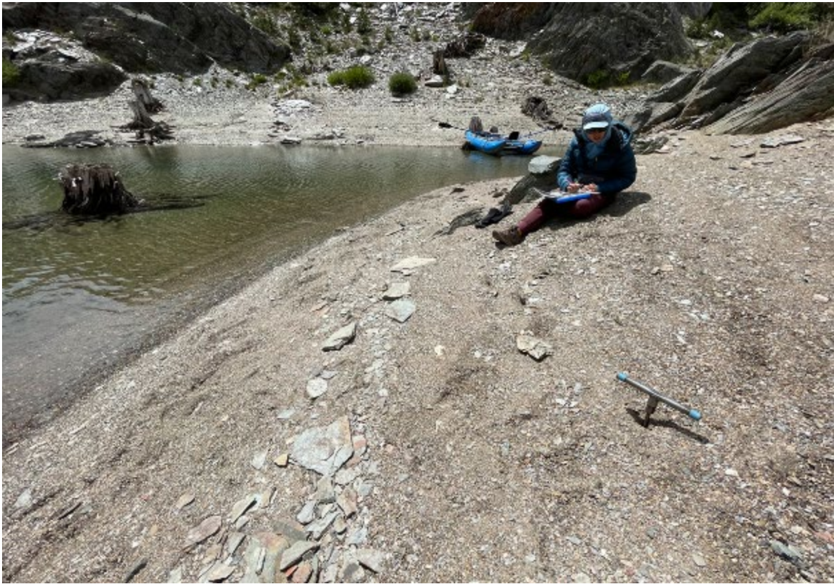
Photo D-3. Cobbley and gravely sand facies mapped along a northern shoreline cove within the secondary basin of Gem Lake indicating a 4-foot depth on the tile probe.
