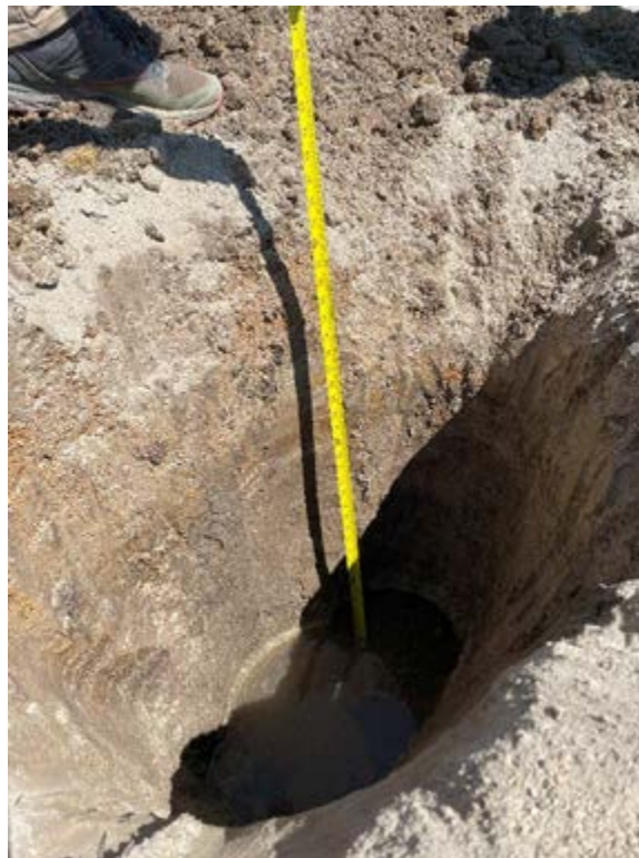
Photo B-4. Waugh 2 contaminant and gradation sample pit. Sample set was broken into two strata.
