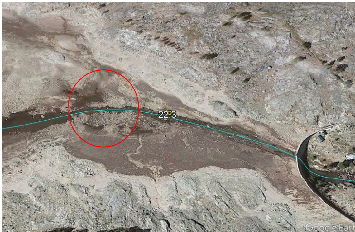
Figure D-1. Boulder and cobble grade break and control located approximately 400 feet upstream of Rush Meadows Dam that along with the presence of shallow bedrock ridges would likely inhibit downcutting of Rush Creek due to dam removal.
