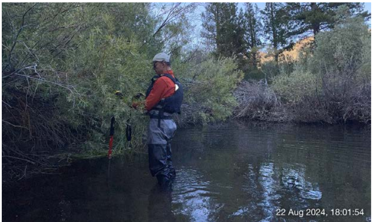
Photo B-39. Reference 5 contaminant and gradation sample collected on left bank low gradient bend where finer sediment deposition was apparent.
