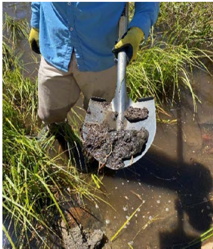
Photo B-27. Agnew 2 remaining contaminant and gradation sample extracted with a shovel below surface organic matter.
