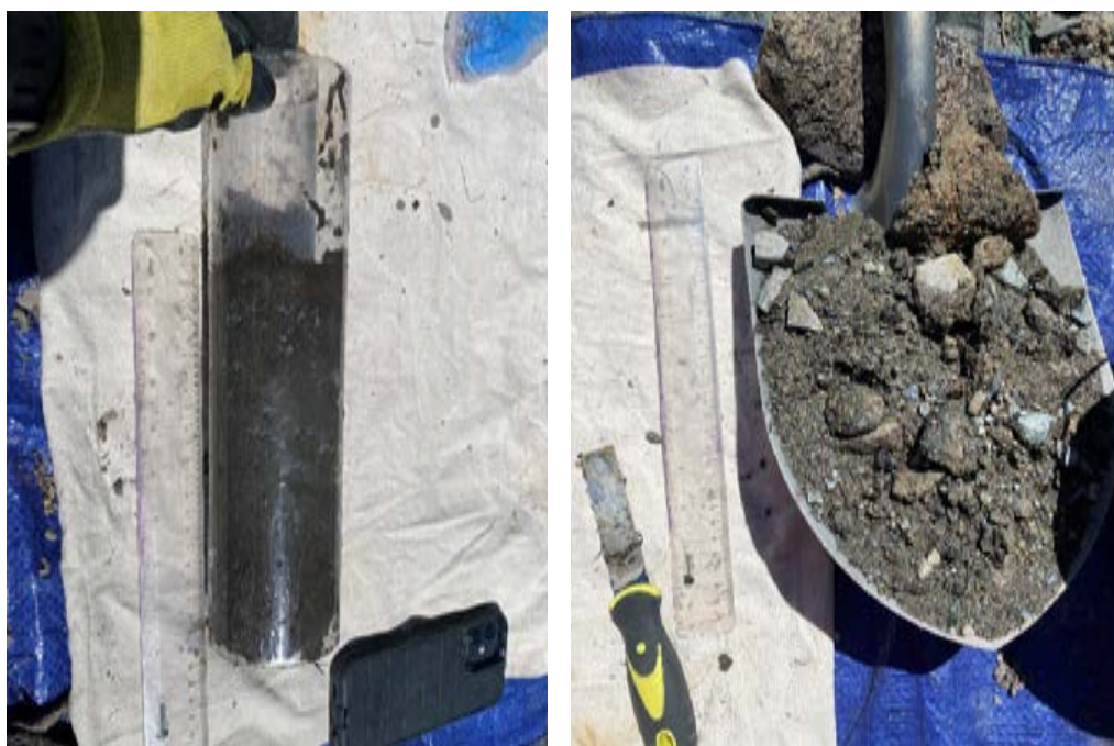
Photo A-23. Agnew 4 Sediment Sample Collected with an AMS Core Sampler and stainless-steel shovel
