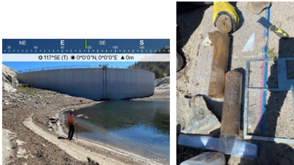
Photo A-12. Waugh 11 Sediment Sample Collected with an AMS Core Sampler Upstream of Dam
