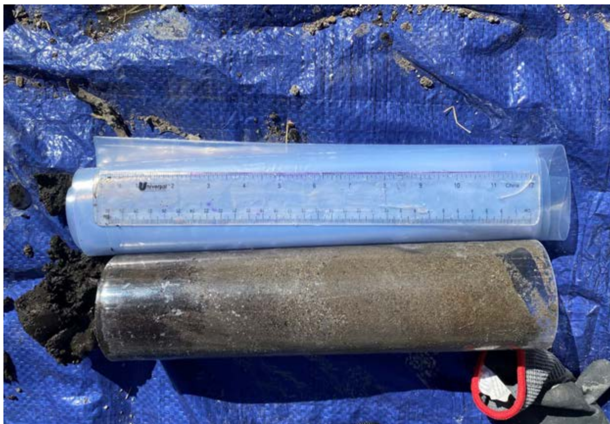
Photo A-21. Agnew 1 Sediment Sample Collected with an AMS Core Sampler
