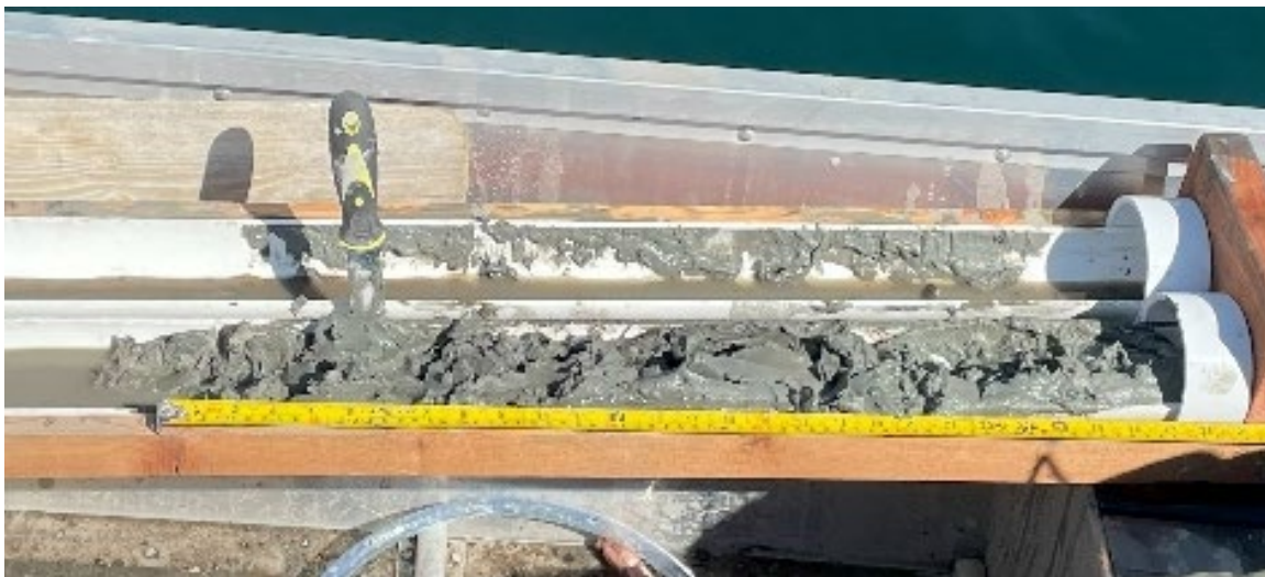
Photo B-14. Gem 1 contaminant and gradation core sample extracted with aluminum core sleeve.
