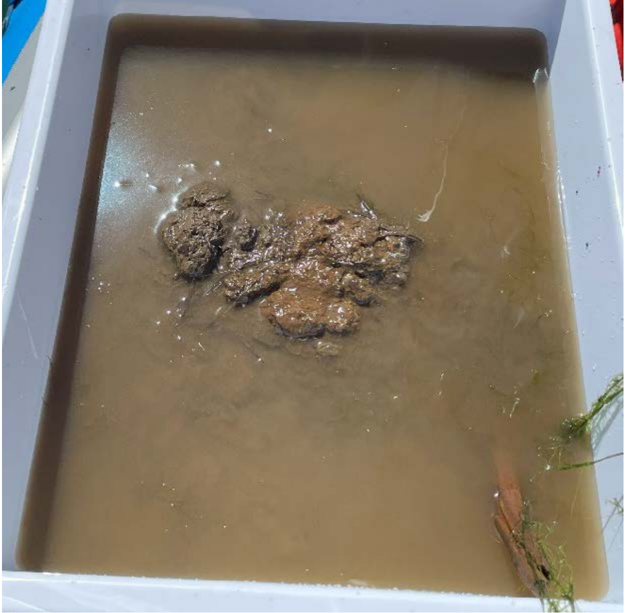
Photo B-21. Gem 7 gradation sample extracted with Ponar grab sampler.
