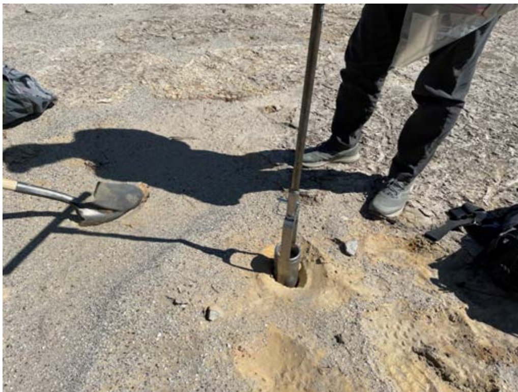
Photo A-7. Waugh 5 Sediment Sample Collected with an AMS Core Sampler
