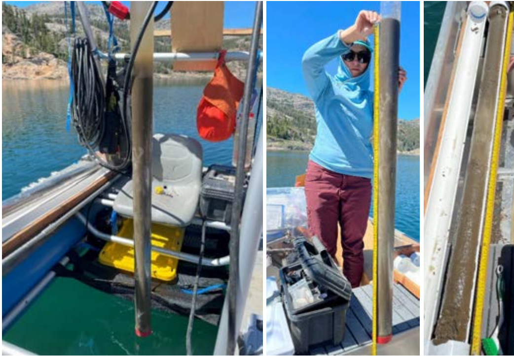
Photo B-17. Gem 3 contaminant and gradation core sample extracted with plastic core sleeve (left and middle) and aluminum sleeve (right).
