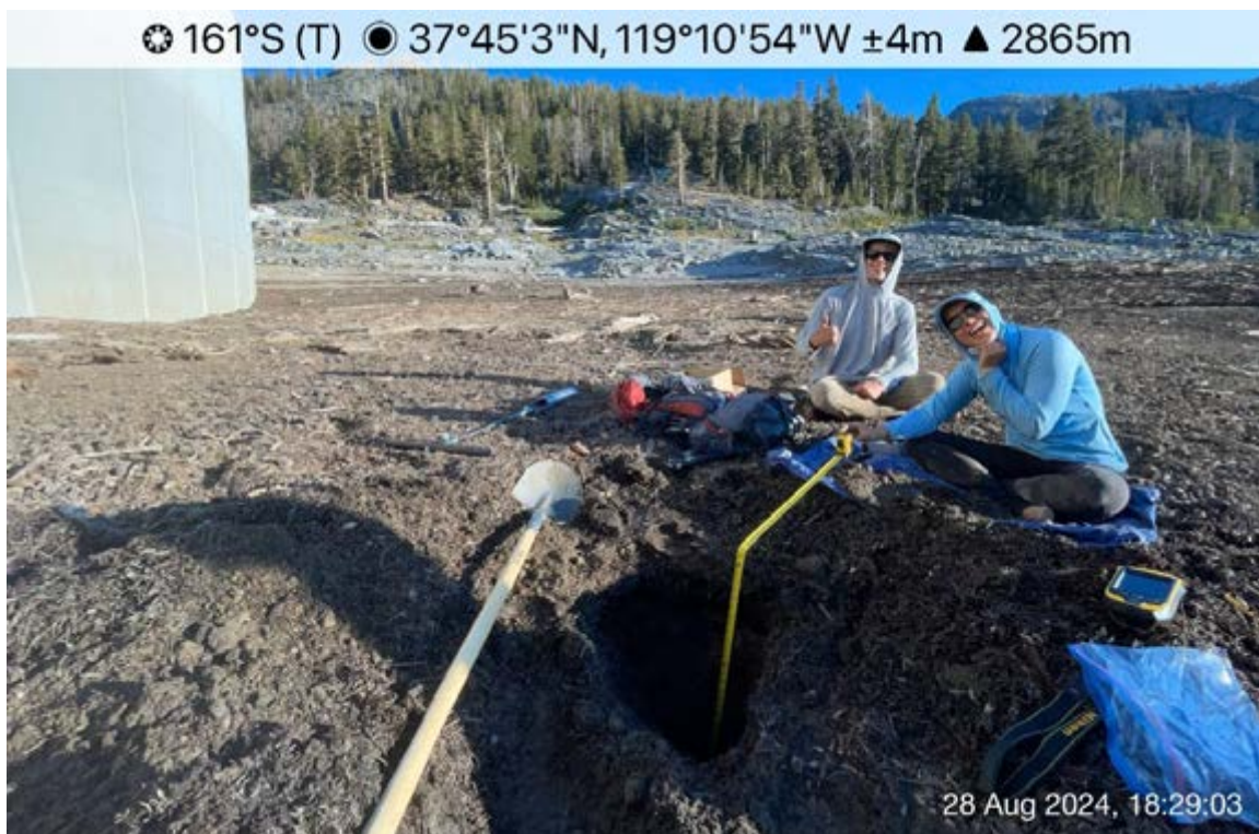
Photo B-12. Waugh 12 contaminant and gradation sample location and pit.
