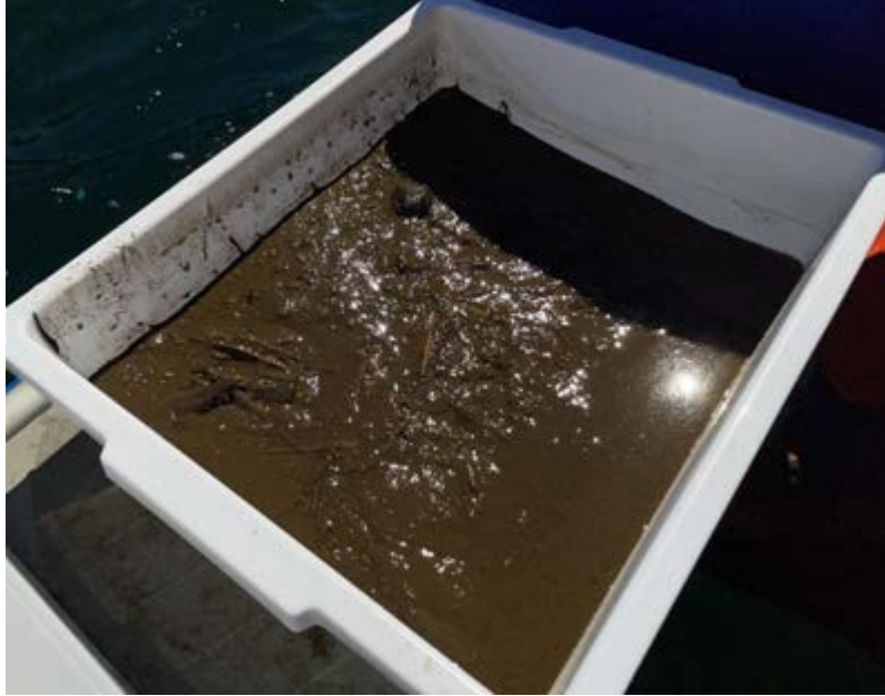
Photo A-20. Gem 7 Sediment Sample Collected with a Standard Ponar
