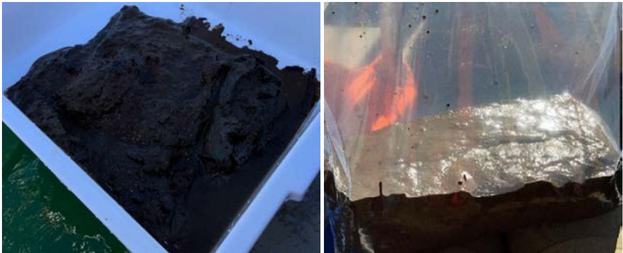
Photo B-20. Gem 6 gradation sample extracted with Ponar grab sampler.
