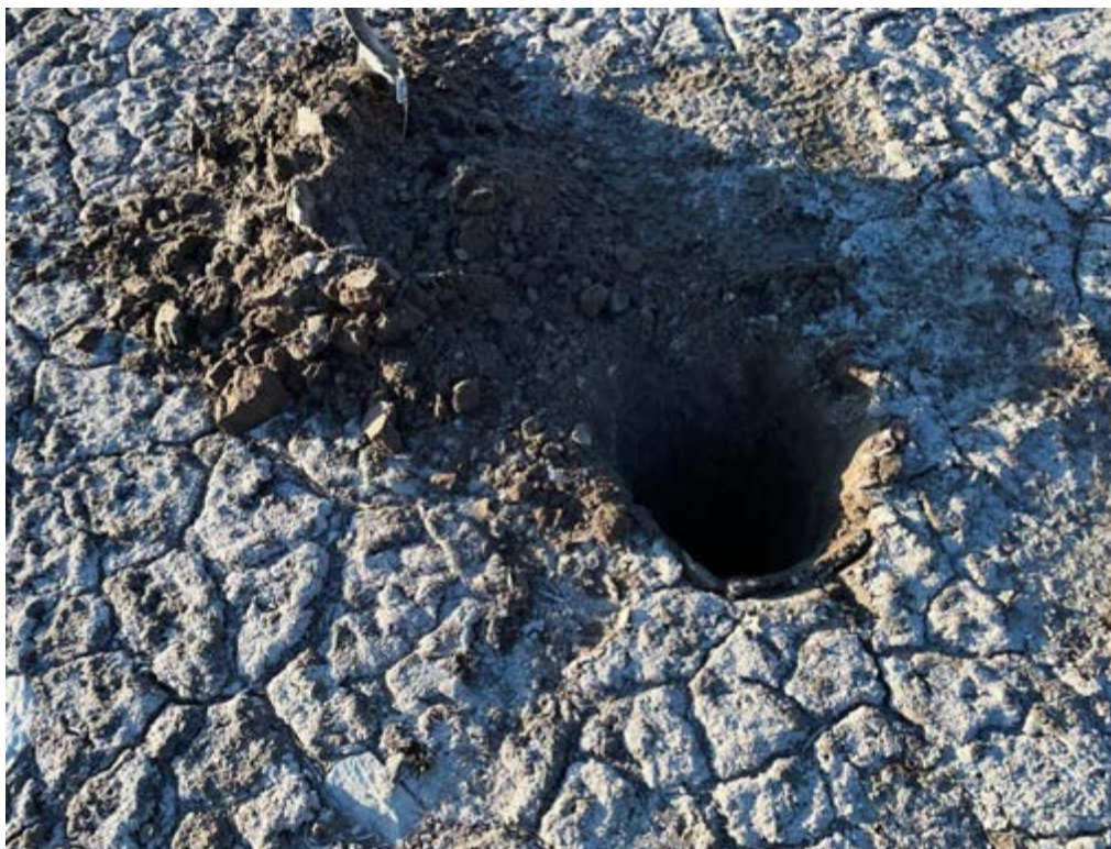
Photo A-11. Waugh 10 Sediment Sample Collected in reservoir accumulation zone upstream of dam.
