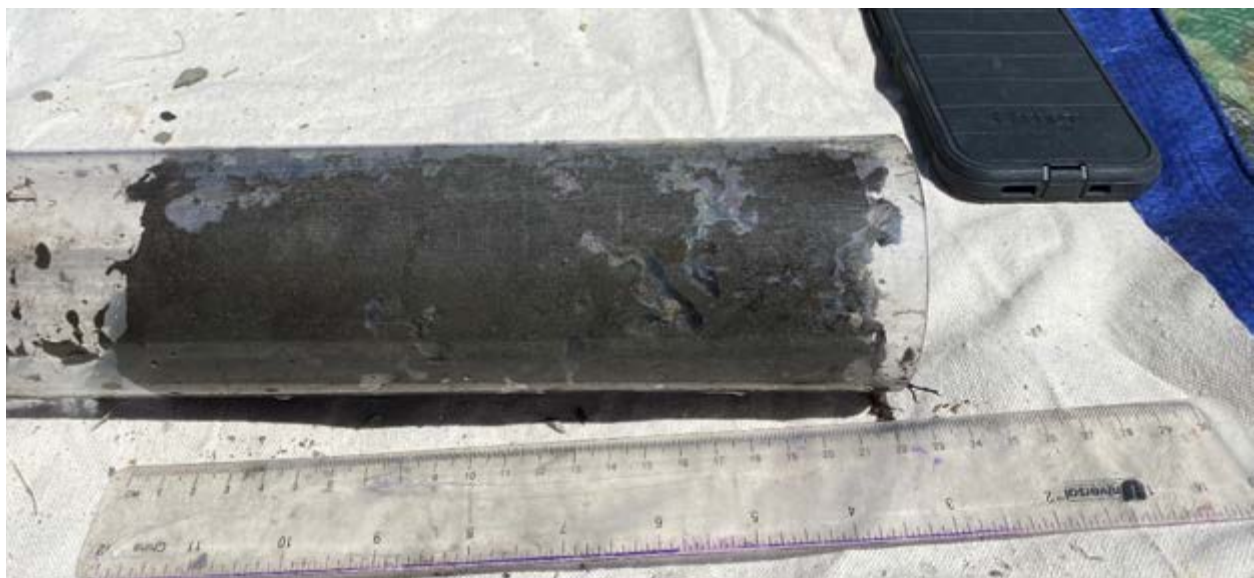
Photo B-31. Agnew 4 contaminant and gradation sample extracted using plastic core sleeve.
