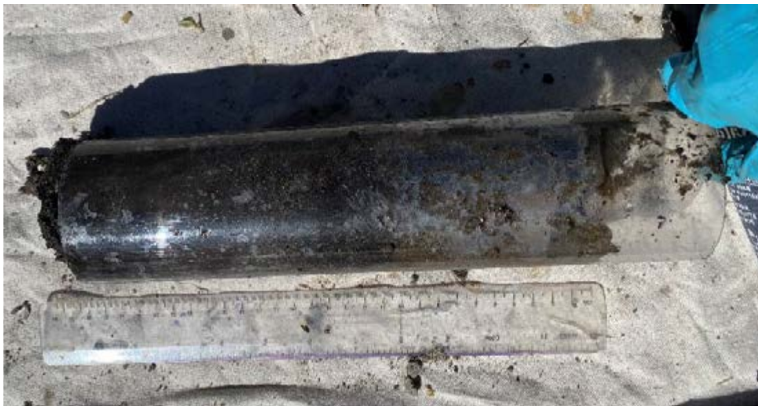
Photo B-29. Agnew 3 contaminant and gradation sample extracted using plastic core sleeve.
