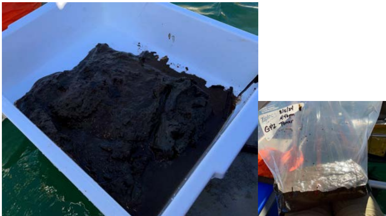
Photo A-19. Gem 6 Sediment Sample Collected with a Standard Ponar
