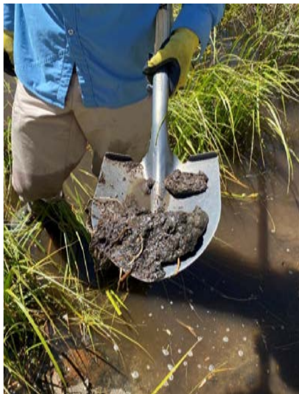
Photo A-21. Agnew 2 Sediment Sample Collected with an AMS Core Sampler and stainless-steel shovel.
