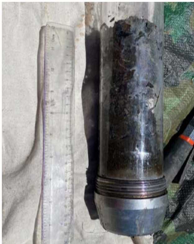
Photo A-21. Agnew 2 Sediment Sample Collected with an AMS Core Sampler and stainless-steel shovel.
