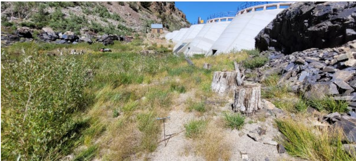
Photo D-4. Bouldery sand facies mapped on the right abutment side of Agnew Dam with a 2.5-foot sediment depth measured with the tile probe.
