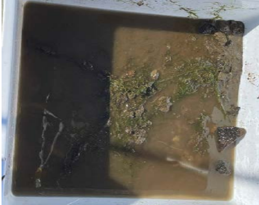
Photo B-15. Gem 1 contaminant and gradation sample extracted with standard Ponar grab sampler.
