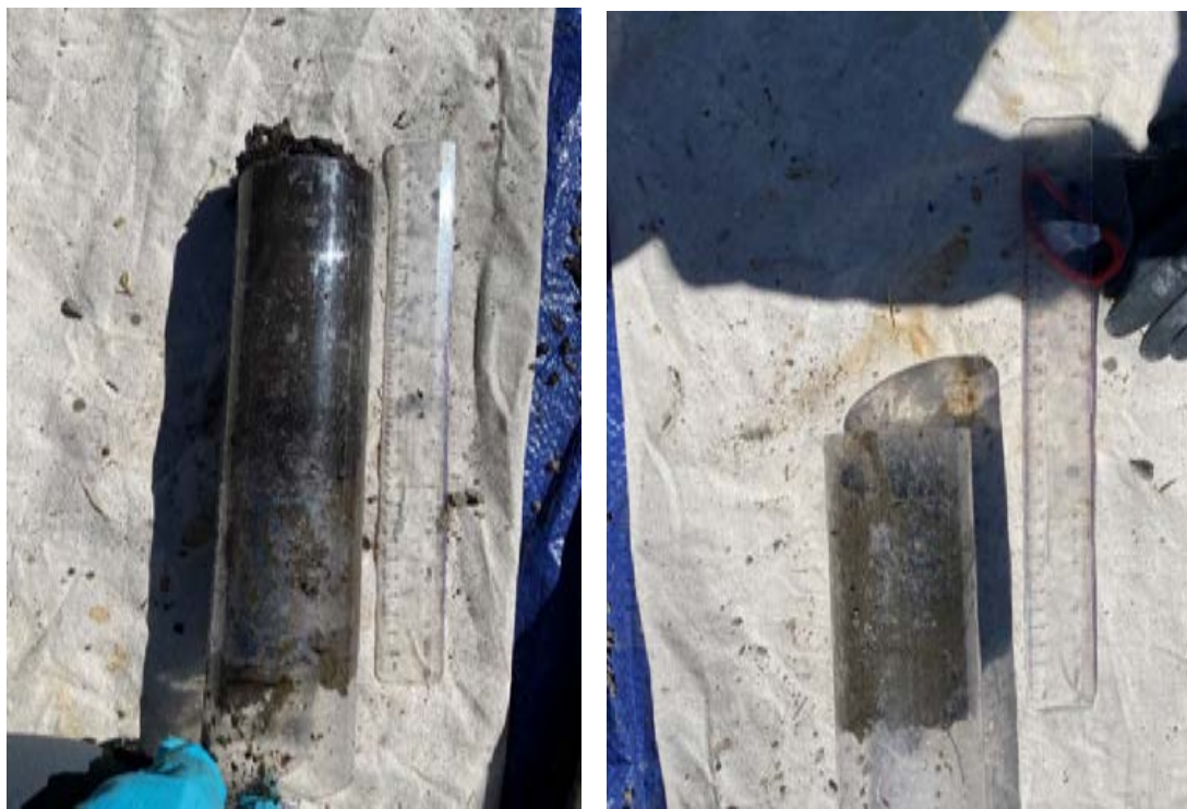
Photo A-22. Agnew 3 Sediment Sample Collected with an AMS Core Sampler.
