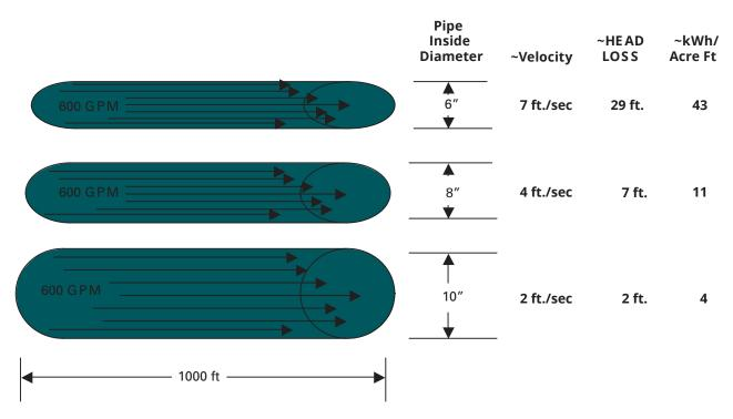
\*\*HAZEN - WILLIAMS METHOD FOR DETERMINING FRICTION LOSS. IRON PIPE = 130 FRICTION COEFFICIENT
