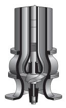
Axial Flow impellers are typically used in agriculture in canal lift pumps, where water flows in a straight line. They provide very high flows at relatively low pressure.
