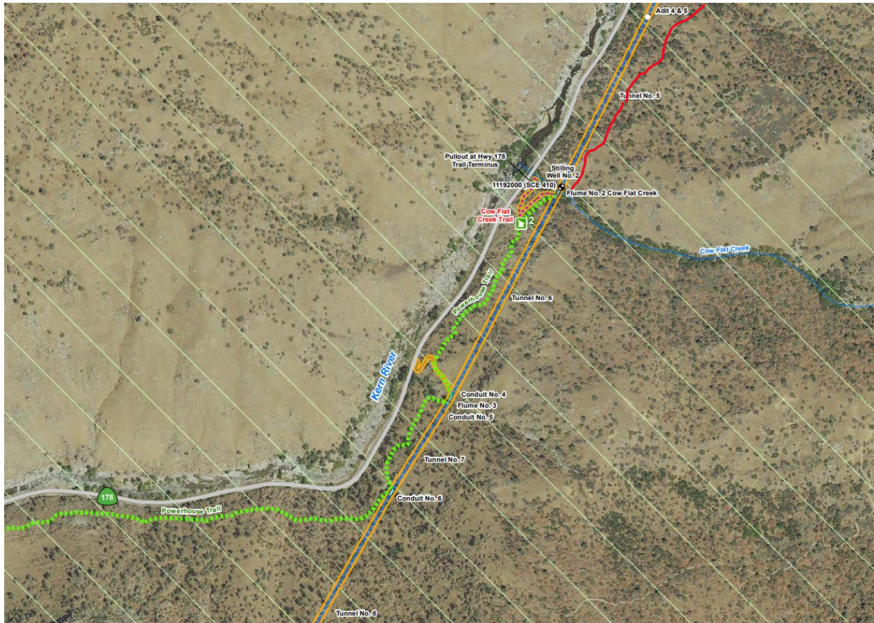
Figure 1. Map from REC-2 TM (p. 50) showing the Cow Flat Creek Trail and the start of the USFS Powerhouse Trail. The Powerhouse Trail connects to KR1 flowline tunnel access points; tunnel tailings visible in talus piles below the trail indicate construction associated with KR1. Red lines show the proposed Kern Gateway Trail alignment continuing upstream of Cow Flat Creek toward Democrat Dam. (Source: SCE REC-2 TM, December 2025; KGT overlay by Kern Gateway Trail Committee)
