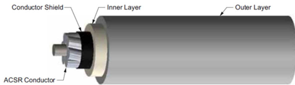
Figure II-5 Three-Layer Covered Conductor Design and Installation
