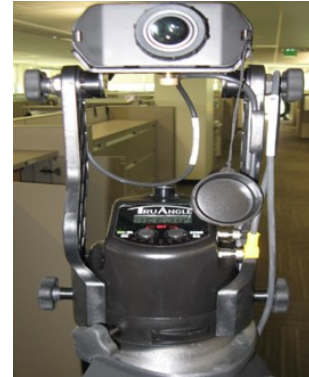
Figure 7.3: Mounted with TruPulse 360R
