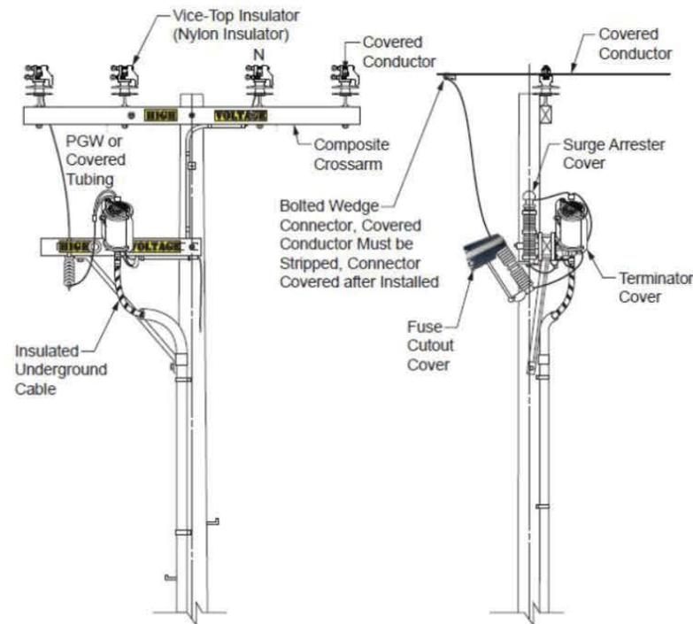
Same concept for three-wire and two-wire constructions
