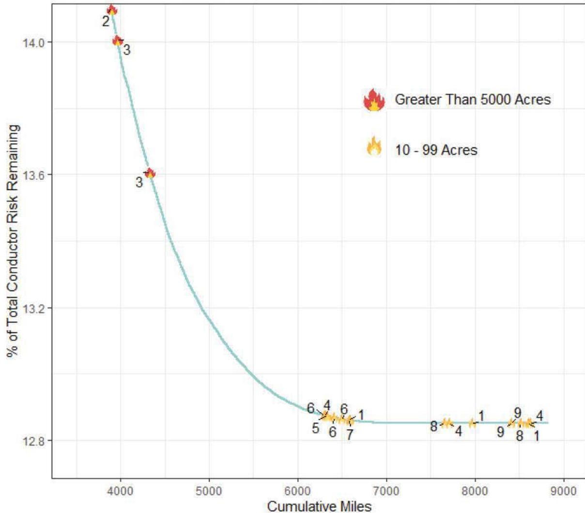
In the graph above, SCE plotted the previously shown nine ignitions along the covered conductor risk buydown curve. The y-axis has been re-labeled from “Percent Remaining Risk” to “% of Total Conductor Risk Remaining,” to reflect the wildfire risk that covered conductor is mitigating, specifically conductor-related risk as opposed to total risk (e.g., risk from a transformer failure).
