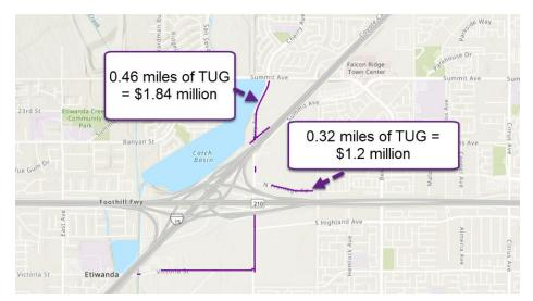
FIGURE 9 - TUG SEGMENTS OF ACOSTA 12KV
