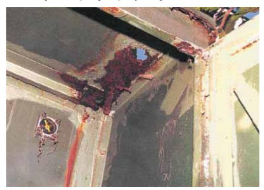
Figure 6–2: Very Heavy Corrosion of Locking Assembly
