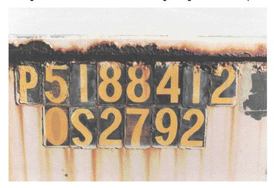
Figure 6–15: Loss of Metal
