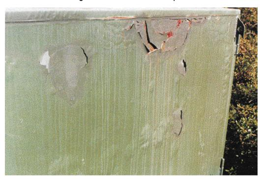
Figure 6–13: Significant Blistering of Paint
