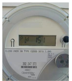
Pid Channel: Program ID Mode- identifies if meter captures usage hourly or every 15 min
