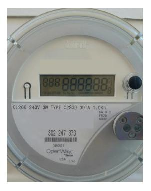
Smart Connect meter cycles through a few different screens. Each Screen displays for 5 seconds. <u>DISPLAY TEST</u>: Self-Test mode. Ensures meter's display is working correctly.
