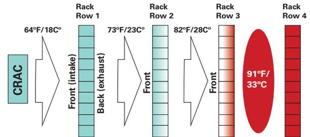
But if several rows are set up in the same orientation, the second row of racks takes in hot exhaust air from the first row. The problem is magnified with each progressive row, as the air temperature becomes hotter, causing more energy usage from A/C to keep the data center cool.
