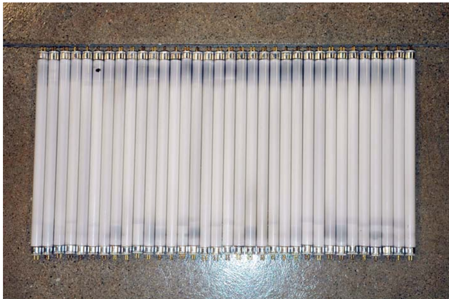
Figure PF-8: Blackened Ends of Failed F8T5 and F13T5 Lamps
