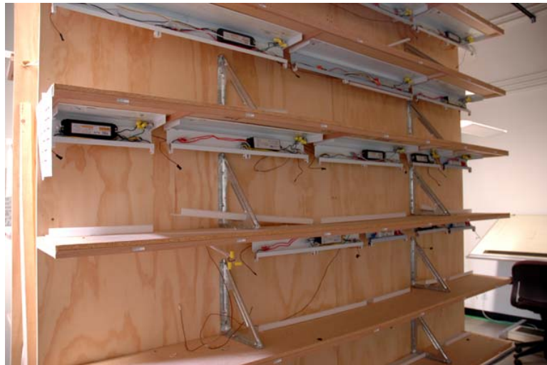
Figure PF-10: T5 Under-Cabinet Test Rack Lamp and Ballast Analysis
