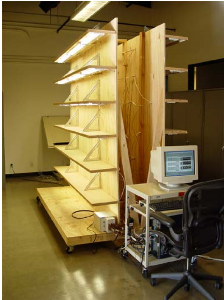
Figure PF-2: T5 Under-Cabinet Test Rack and Instrumentation System
