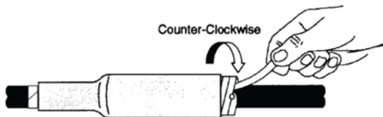
Figure CC 170-7: Cold Shrink Application
