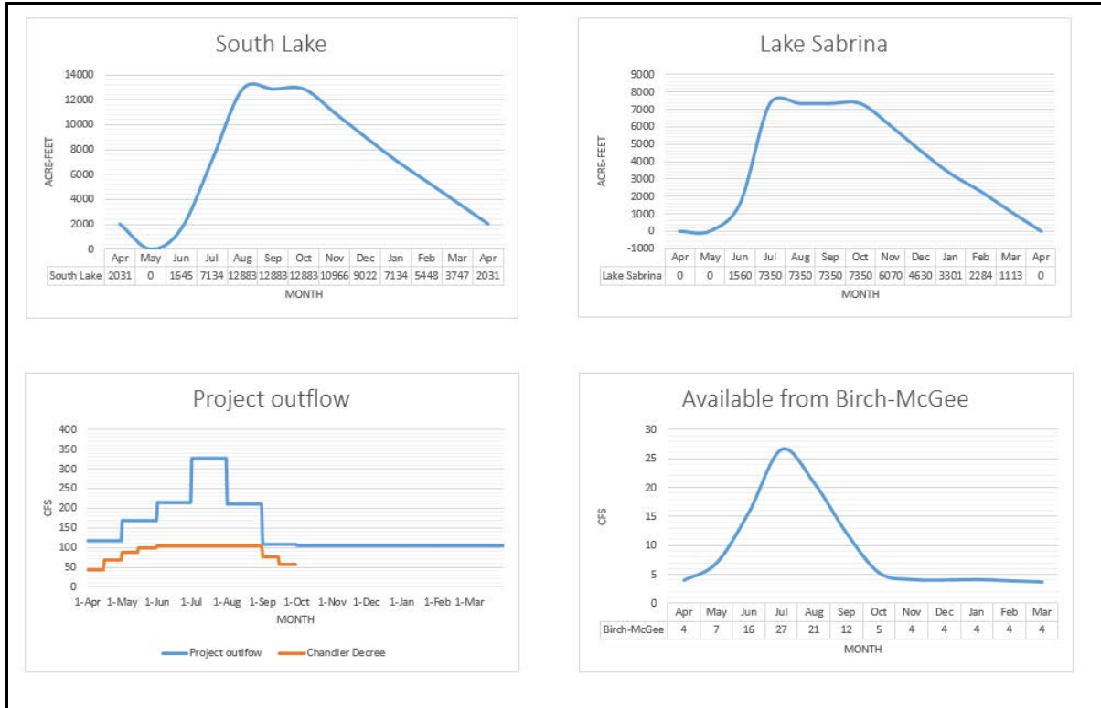
FIGURE 3-5 OPERATING RULE CURVE – HIGH WATER YEAR
